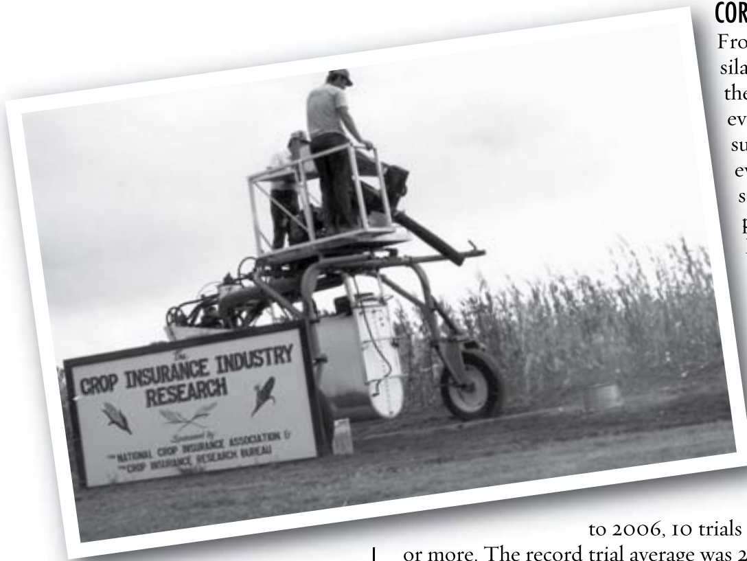
Demonstration of the "hail machine" that was used to simulate hail damage to corn and other crops to evaluate yield losses due to hail damage.
