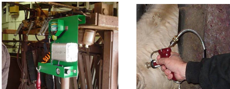
Figure 1. Felton Pneumatic System and needle-free injector.
