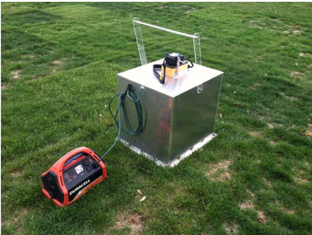
Figure 2. The light box, powered by the portable pack, in use over a research plot.
