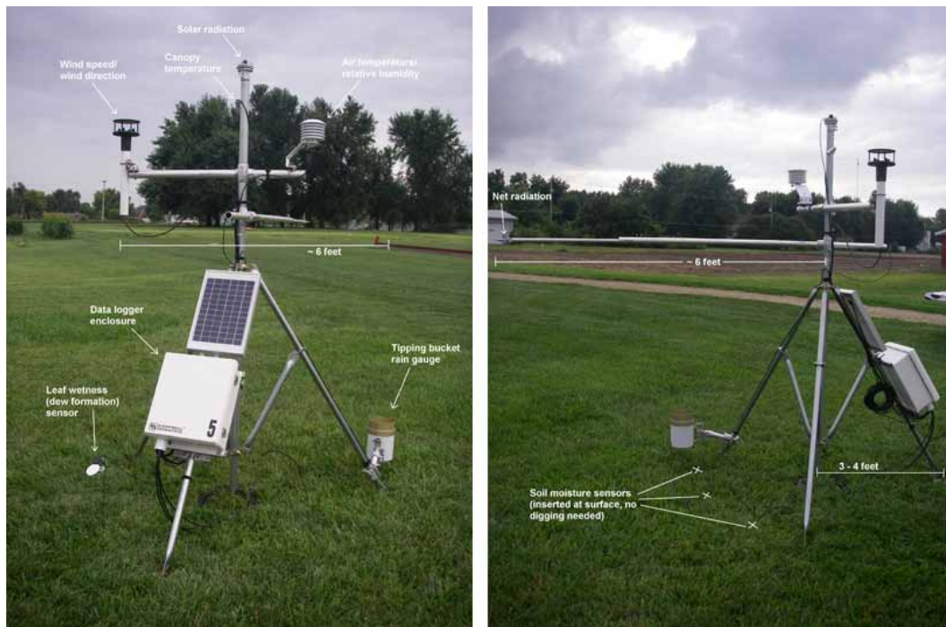
Figure 1. Schematic of the small tripod-mounted weather stations deployed in residential lawns.
