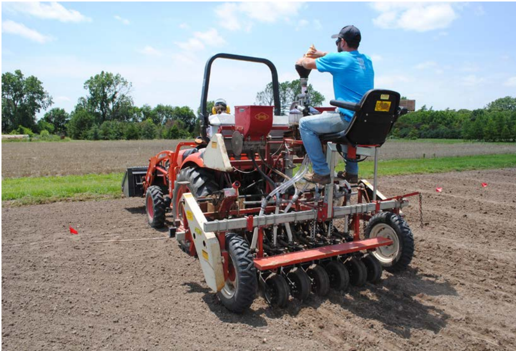
Figure 3. Hege 1000 grain drill for planting hemp variety plots.
