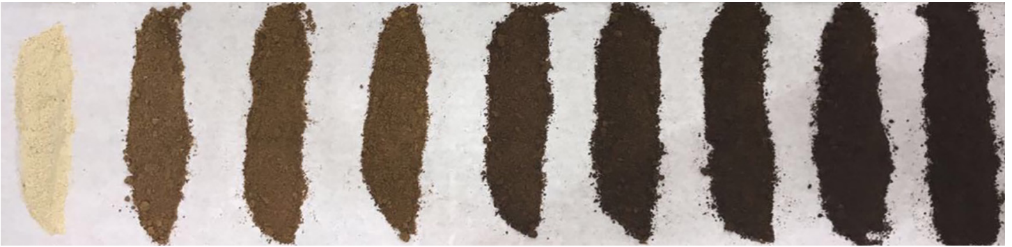
Figure 1. Ground soy white flakes exposed to an autoclave at 262°F for 0, 5, 10, 15, 30, 45, and 60 min at 29 PSI, simulating the heat step in soybean meal processing to create a range of soybean meal quality.
