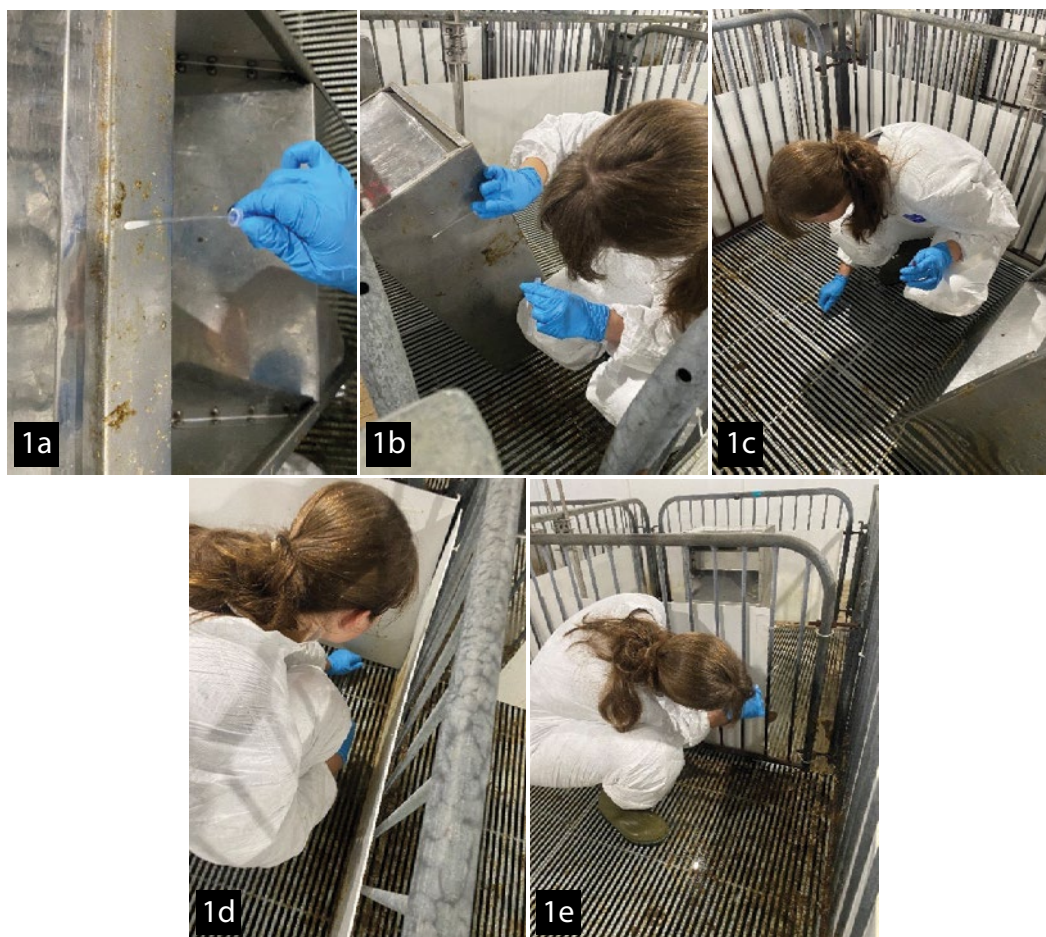
Figure 1. 1a) Sampling of the central outer lip of the pen feeder with the UltraSnap surface ATP Test (Hygenia, Camarillo, CA); 1b) Sampling of exterior side of inverted feeder with the UltraSnap surface ATP Test; 1c) Sampling of center paneling of triangular bar flooring in pen; 1d) Sampling of right back corner paneling of triangular bar flooring in pen; 1e) Sampling of corner wall solid plastic pen divider in between metal bars of pen.
