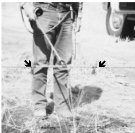
Figure 1. Spray rig used to apply herbicides over the seedlings. The nozzle positions allowed application to the side of seedlings.
