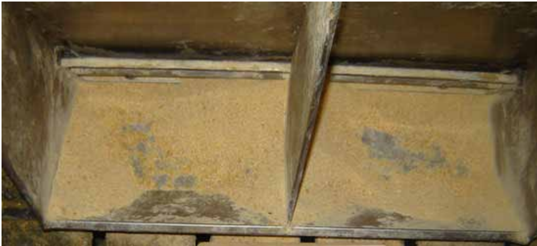
Figure 2. Wide feeder adjustment (minimum feeder-gap opening was 1.00 in. with a maximum gap of 1.25 in.) averaged 83% feeder pan coverage.
