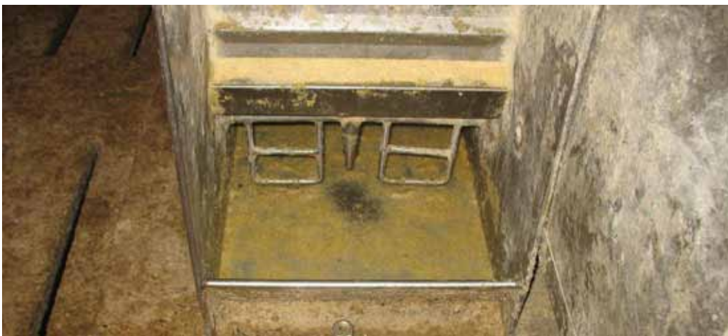
Figure 3. Wet-dry feeder at setting 14 with a 1.00-in. opening and \approx 65\% pan coverage.
