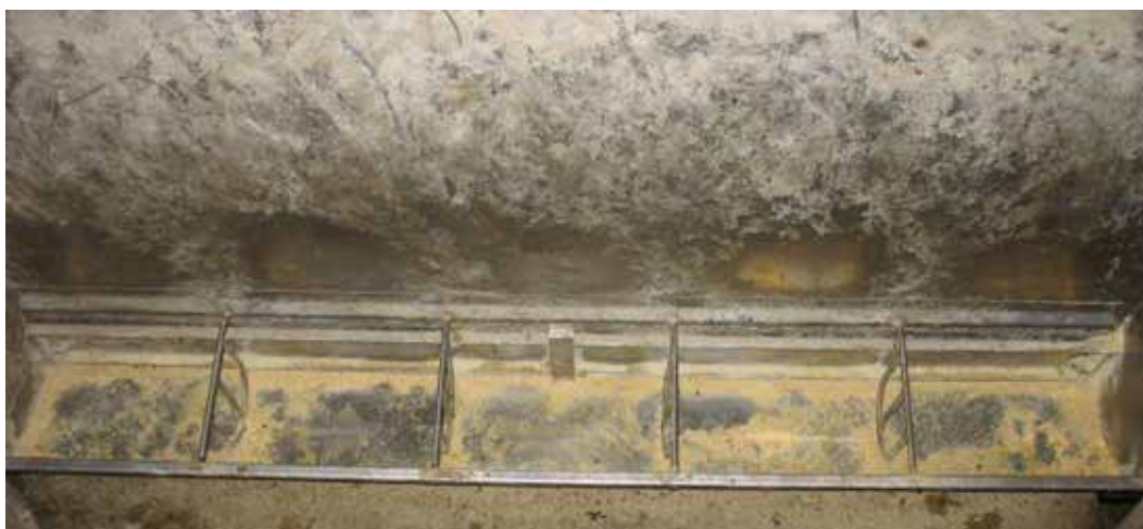
Figure 8. Conventional dry feeder at setting 6 with a 0.58- to 0.82-in. opening and \approx 27\% pan coverage.
