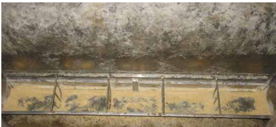
Figure 9. Conventional dry feeder at setting 8 with a 0.83- to 1.12-in. opening and \approx 57\% pan coverage.
