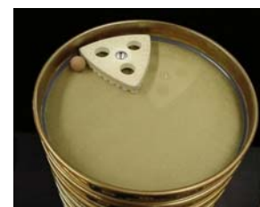
Figure 2. Ball and Brush Resting of a Sieve.
