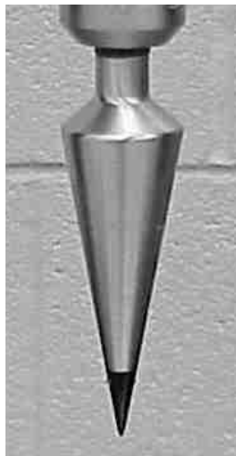
Figure 3. Plumb Bob Probe
